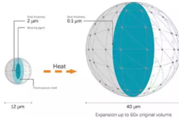
for lightweight solutions. Since reducing weight contributes very well to the fuel efficiency in vehicles, these microspheres could be a great advantage in the areas where weight reduction is important.
