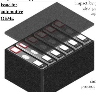
LASTAN™ is a non-mineral flame-resistant fabric made by air baking a special acrylic fiber at 200 −300°C. It is characterized by high flame resistance and good electrical insulation, which are further improved by a special coating process that also augments abrasion resistance. This allows the material to provide effective protection against particle bombardment from venting gas.
