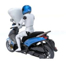
Through virtual and physical testing, we have demonstrated the benefit of the airbag in frontal crashes, and we acknowledge that there is a need for additional solutions to
