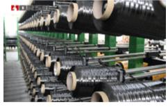
Toray began the commercial production of TORAY-CA™ carbon fiber in 1971 at the Ehime Plant and diver-
