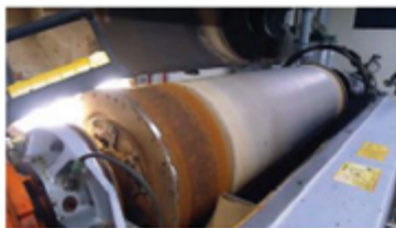
Centrifuge before adding scale inhibitor
